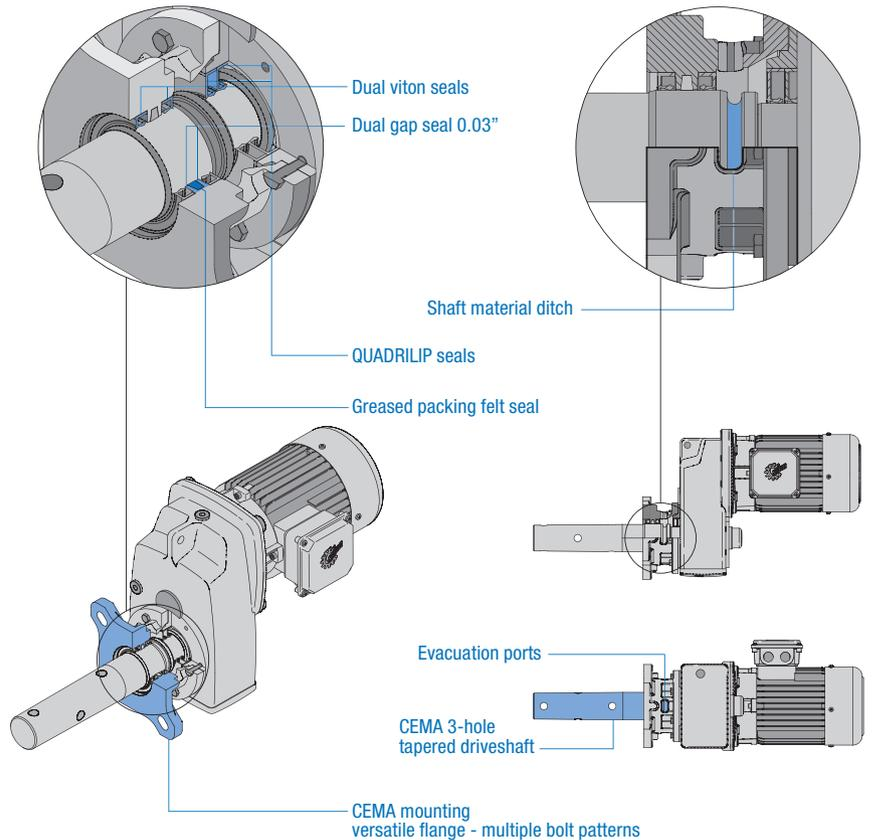
The screw conveyor package is available for both CLINCHER™ parallel shaft gear units and right-angle helical bevel gear units. The CEMA flange and shaft assembly are a unique NORD design to offer superior protection against unwanted debris.
