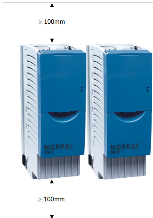
Fig. 1 Mounting distances for SK 5xxE
