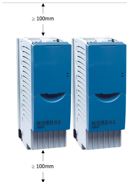
Fig. 1 Mounting distances for SK 5xxE
