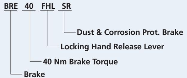
Brake, 40 Nm with a locking hand release lever and dust & corrosion protected brake.
