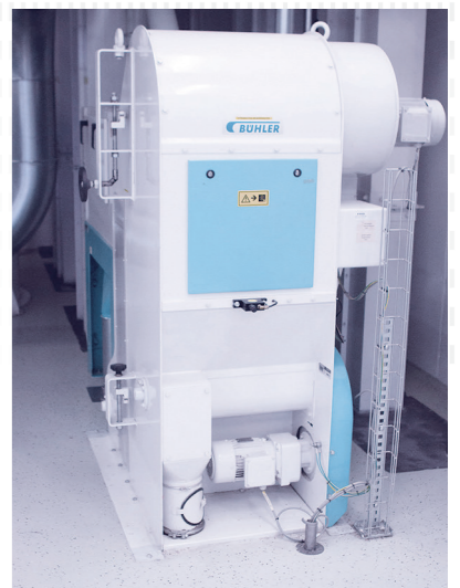
Grain cleaner NORD driven screw conveyor removes low-density fraction in air-recycling aspirator
