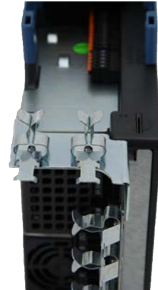
Detailed view of mounted EMC kits
