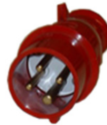
CEE three-phase plug 16 A, 400 V, 3L+N+PE, 6h, IP44
