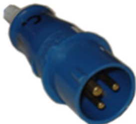
CEE alternating current plug 16 A, 230 V, L+N+PE, 6h, IP44
