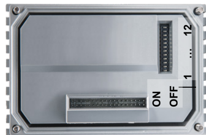
Factory settings DIP switches: OFF
